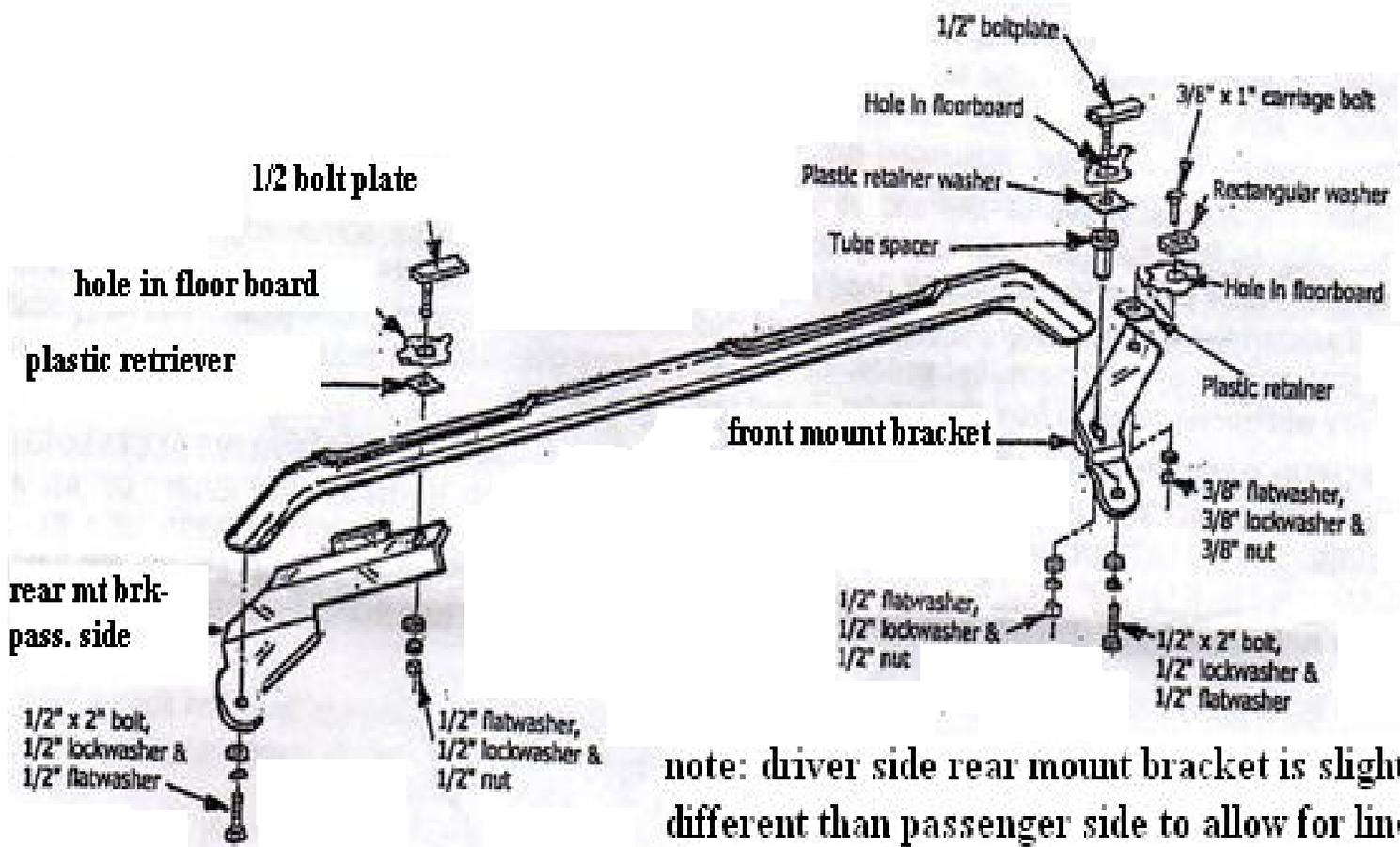
**note: driver side rear mount bracket is slightly different than passenger side to allow for line clearance**
