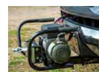
Allows a winch to be easily attached to a receiver
