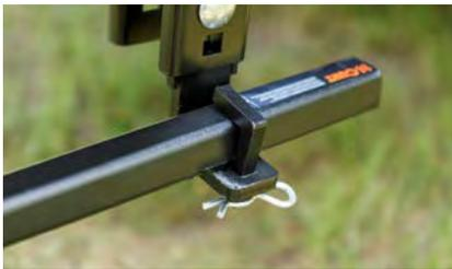
Two points of sway control use friction to distribute weight evenly, keeping trailer aligned
