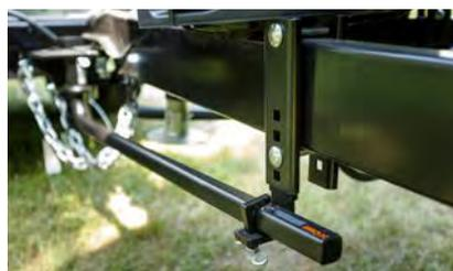
Heavy-duty, adjustable support brackets provide two points of passive sway control
