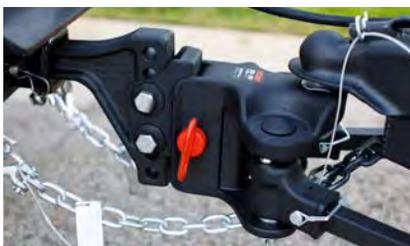
Head-tilt adjustment feature provides 15° of adjustment for precise leveling
