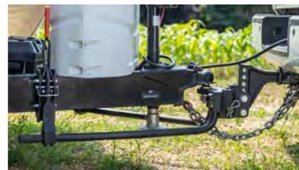
Spring-loaded bars leverage trailer weight and spread it across all axles evenly
