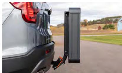
Carrier can be flipped in the shank when not carrying a load for compact transport
