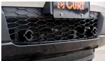
Our simplified base plate designs provide improved fitment on each vehicle, requiring fewer front-end modifications and no extra trimming for RV harness installation
