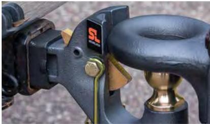
As you back up the vehicle, a built-in back plate helps position the coupler or lunette ring for easier hookup
