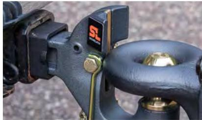
As the coupler is lowered onto the pintle hitch, SecureLatch automatically locks without any manual coupling required
