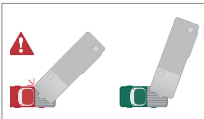
Provides 12" of displacement for the coupling point, adding turning clearance for short-bed trucks and avoiding trailer obstruction
