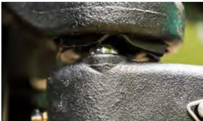
Lateral forces compress the bearings into a rotational groove to actively resist sway. The larger the sway event, the greater the resistance applied by the WD hitch
