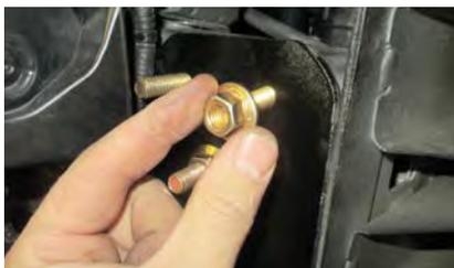
Large 1/4" thick spacers better distribute weight. Superior grade-8 hardware, serrated hex flange nuts and fishwire are included for easy installation from inside the frame
