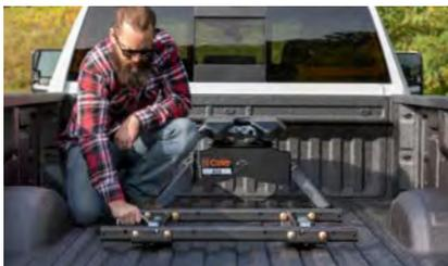
Easily transfer existing hitch from previous truck to new puck-equipped truck
