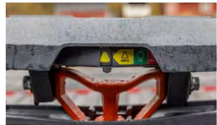
Three-position coupling indicator clearly shows coupling status
