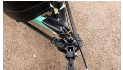
During turns the bearings compress, allowing them to rotate freely. Afterwards they return to their tensioned, home position
