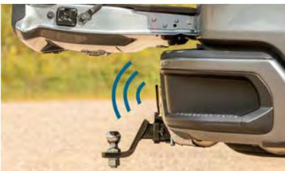
Prevents deployment of inner tailgate panel when ball mount is installed
