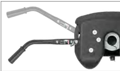
Lockable handle self-resets to the ready-to-couple position after the hitch is uncoupled
