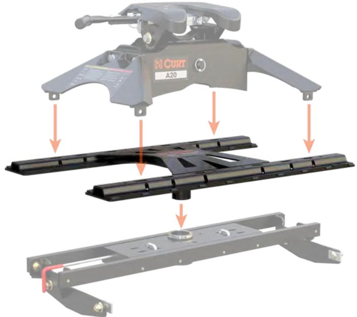
**Step 1 - Pick a gooseneck hitch. If your customer has a gooseneck hitch, see step 2**
