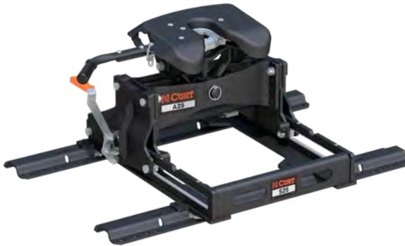
16651 - A25 head with S25 slider and base rails
