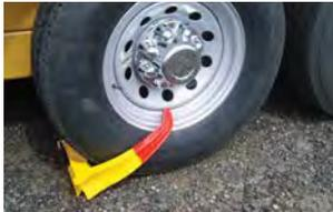
Secures unattended trailers or vehicles by clamping on the wheel
