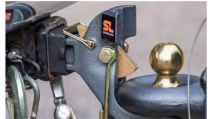
Finally, insert the secondary safety pin, connect the safety chains and you're ready to tow with confidence and without chucking
