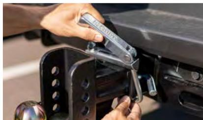
No-tool installation and easy-to-adjust clamp lever (clamp-style)
