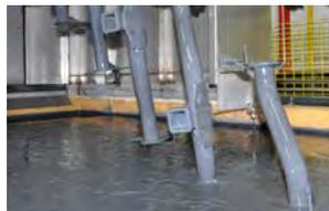
A-coat applied inside and out and co-cured with powder coat for maximum rust resistance
