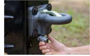
Drop-in pin accepts lock to deter theft (turns 90° while coupled)
