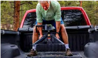
65% lighter than most traditional 5th wheel hitches (main body weighs up to 70 lbs.)
