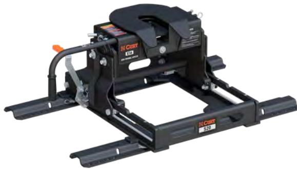
16611 - E16 head with S20 slider and base rails
