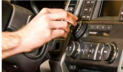
Clean, dash-mounted, OEM-style user interface with 10 tri-color LEDs
