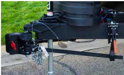
Upward force on the ends of the spring bars tensions the bearings, directing them towards the 'home' position, increasing sway control
