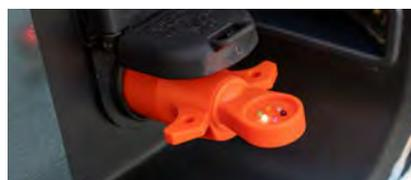
Color-coded LEDs to easily distinguish each vehicle signal (#58272, #58273)
