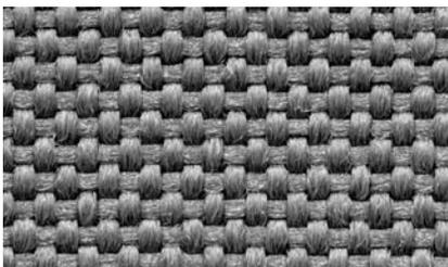
Top is made of durable, woven 600-denier terylene fabric to keep spills and dirt out
